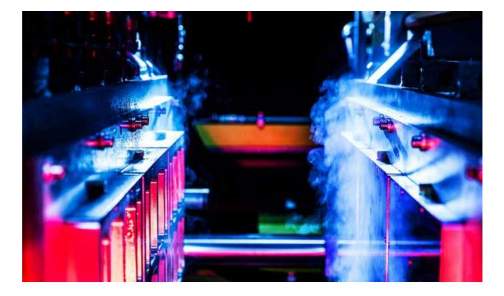
In just a few seconds, Speedfactory machines can heat and mold material into Adidas' running shoe soles, with a single worker required to wedge in pieces of plastic. Manual stitching and gluing are replaced with molding and bonding done by machines to roll out shoes in a day. Sneakers can also be customized by style and fit. More Speedfactories are planned for Atlanta, Paris, London, New York, Los Angeles, Tokyo and Shanghai in 2018.
